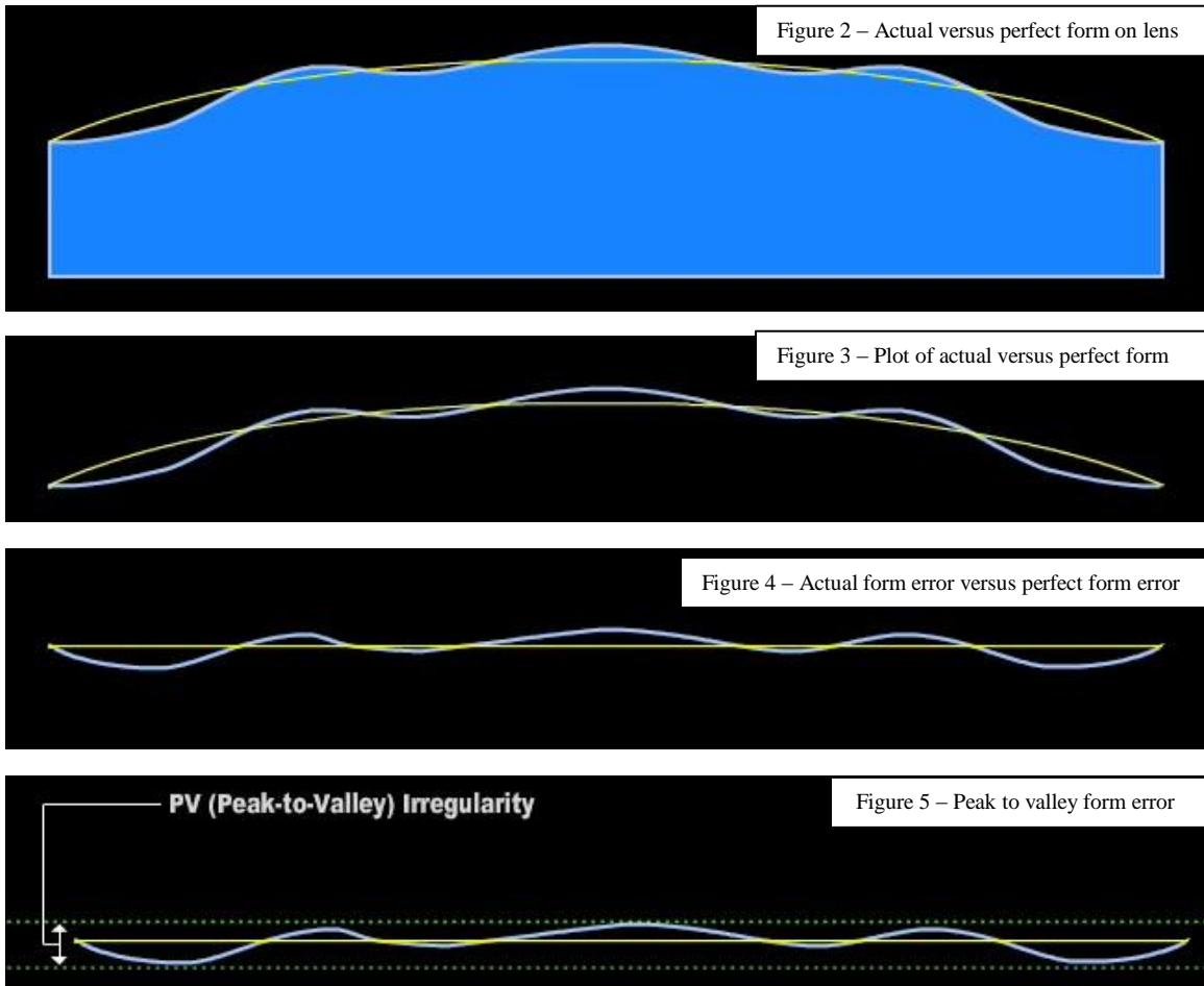
Controlling the rate of change in nonuniform deviation in addition to the magnitude is important to system performance<sup>2</sup>, especially those containing aspheric surfaces.<sup>3</sup> The slopes resulting from midspatial (0.5 – 4mm) frequency errors subaperture polishing may cause can devastate system performance, and applying a maximum slope error specification to the traditional form error can control the contribution.
