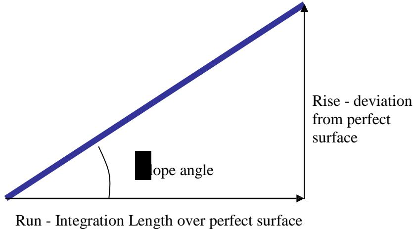
Slope error specification consists of three portions:
