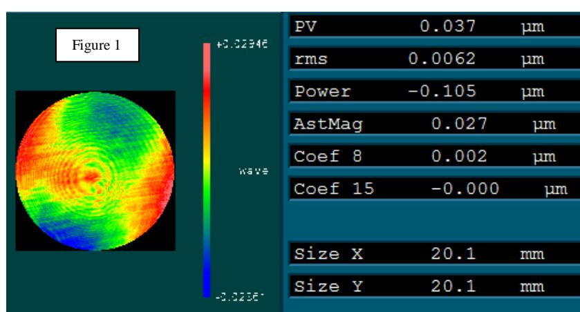
and specifically shows the separation into contributors. The contributions of astigmatism (AstMag), third order spherical aberration (Coef 8) and fifth order spherical aberration (Coef 15) are shown separate from the traditional bundled peak to valley irregularity (PV).
